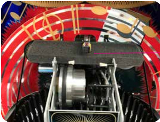
FIG2 : Mechanism in transit mode showing retaining foam
