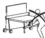
Do not use the crossbeam or legs as support when pulling the release over.
