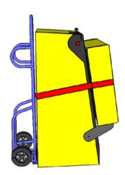
10. Secure all loose parts and transport with a hand truck in the upright position.
